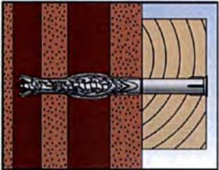
5. Correctly installed anchor in hollow masonry.
