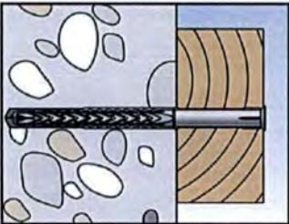
6. Correctly installed anchor in concrete.
